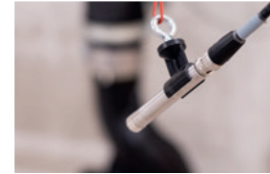
Room acoustic measurement of the radiated airborne sound from a Geberit Silent-db20 Sovent fitting.
